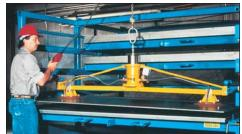
ANVER® Mechanical Vacuum Lifters do not rely on plant power, outside controls, or complex accessories. These self-contained units create their own vacuum mechanically, giving them unmatched versatility for use in metal fabricating plants, service centers, warehouses, and plate yards. These lifters offer instant attach and release via the hoist up and down. The internal piston and rolling diaphragm create vacuum and will work silently with minimum maintenance for years.
